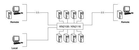
Access to any computer connected to the installation from the local console is easily accomplished either by entering *hotkey* combinations from the keyboard, or by means of a powerful mouse driven OSD (On Screen Display) menu system. A convenient *Auto Scan* feature also permits automatic scanning and monitoring of the activities of all computers running on the installation one by one.
